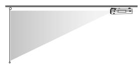
The distance between the projector and the screen determines the actual image size. To determine the exact distance required for a particular image size (or to determine the size of an image at a particular distance), use the following formulas. (Remember that the size of the image can be changed by rotating the zoom ring.)
